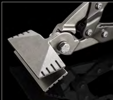
1/4" depth marks on the blades allow for quick bends.
