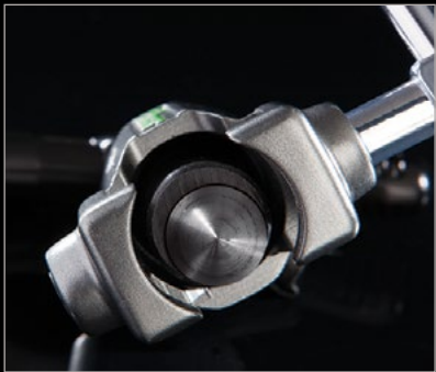
An off-center mounted cone helps to uniformly shape the tube.
