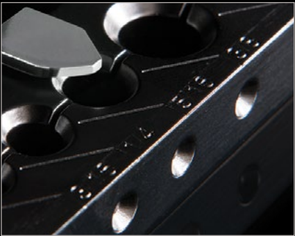
Ball detents ensure proper and precise alignment to guarantee a perfect flare or swage every time.
