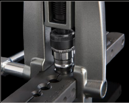
Push down the yoke and with fewer rotations, you get a precise flare or swage.
