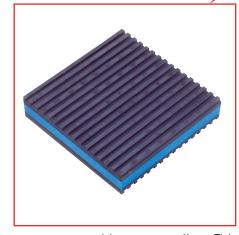
These sheets are laminated in such a way that the ribs are ninety degrees opposed to one-another. This opposition provides a natural resistance to creep or "walking" normally associated with vibrations.
