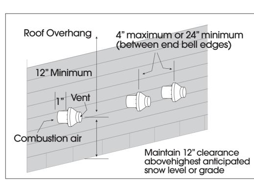
Figure 6-Sidewall Termination for Multiple Horizontal Concentric Vents
