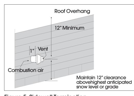
Figure 5-Sidewall Termination
