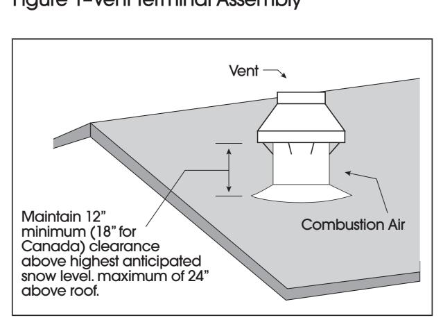
Figure 2-Typical Roof Installation
