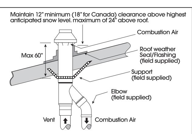
Figure 3-Typical Roof Install
