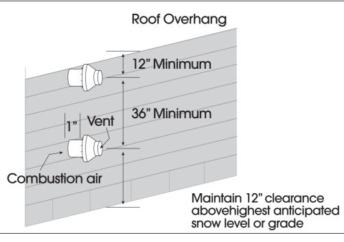
Figure 4-Sidewall Termination for Multiple Vertical Concentric Vents
