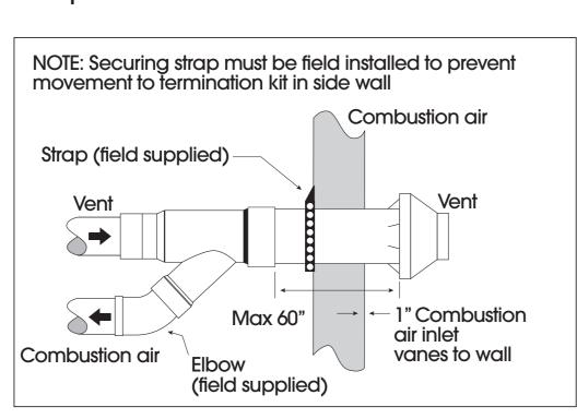
Figure 7-Sidewall Termination Details
