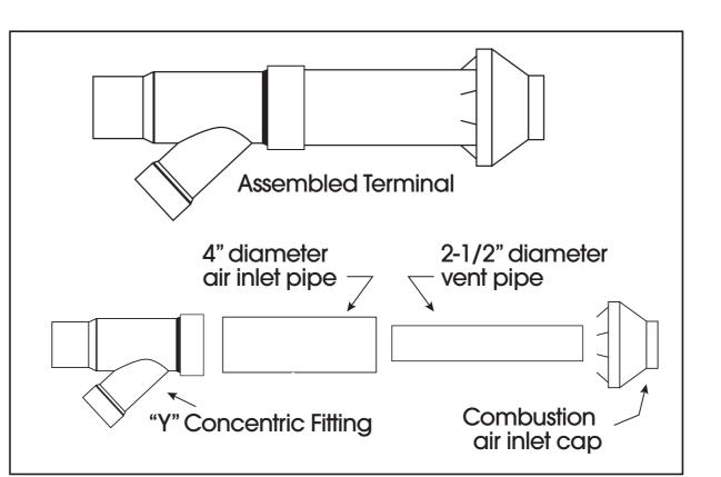
Figure 1-Vent Terminal Assembly
