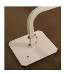
Our VRF Super Stand has four 12" x 12" feet, made from 7-gauge steel and 11-gauge steel tubing. It adjusts in 1/4" and 1/2" increments. This is done by rotating the foot 180 degrees. There are two 1/2" holes in each foot to secure the stand.
