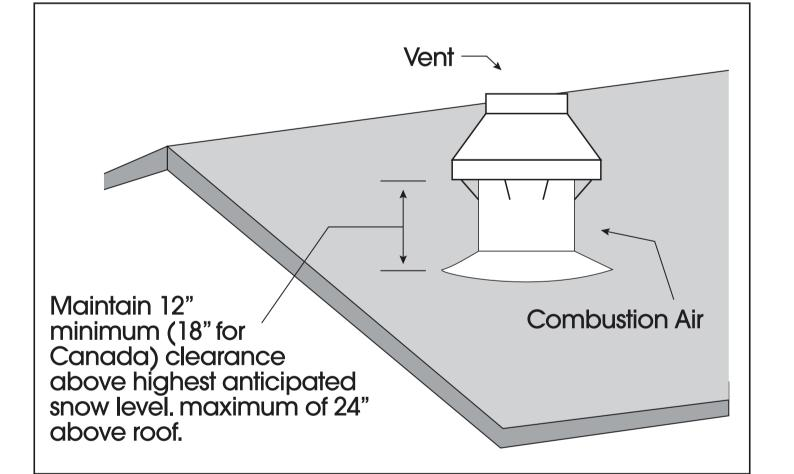
Figure 2-Typical Roof Installation
