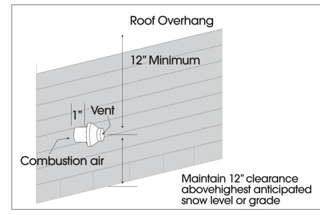
Figure 5–Sidewall Termination
