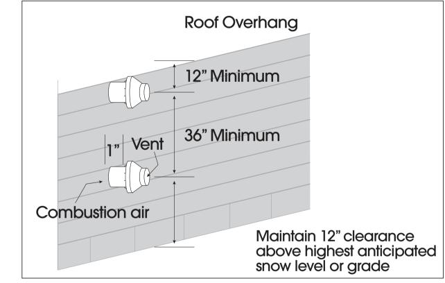
Figure 4–Sidewall Termination for Multiple Vertical Concentric Vents
