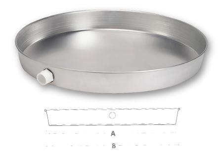
Aluminum water heater pans can be installed under gas or electric water heaters to protect from water damage. Includes a 1" PVC drain fittings to allow for connection to indirect drain. Each pan is manufactured from .032 in. prime aluminum with a pre-cut side opening to accommodate a drain fitting. Pan depth is a minimum 2.5 in.
