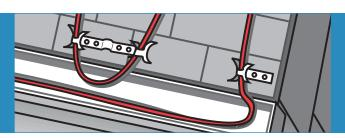
Thermwire®-comp heaters are used to prevent migration of refrigerant into crankcase oil when compressors are operated in cold temperatures. Use of these heaters can prevent excessive wear and loss of refrigerant efficiency.
